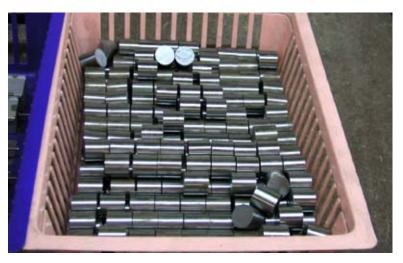
All Royer microphone components are fashioned from solid ingot iron. This is an expensive and painstaking process, but well worth it in the end. Here is a view of R-121 XLR inserts in raw form - solid hunks of iron. It will take many machining operations to produce the finished parts.
