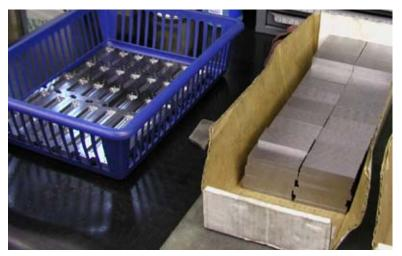
R-121 transducer frames, before and after machining. The transducers start out as a solid block of ingot iron (right view) and after numerous operations can be seen as finished frames on the left. All Royer components are fashioned this way.
