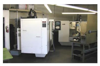
A view of the CNC machine shop, where all Royer microphone parts are manufactured using state-of-the-art CNC machines. Here is a view of two CNC machines that are programmed to produce R-121 transducers and barrels.
