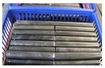
A close up view of rough R-121 barrels. These parts are already rough-cut to length and predrilled. Slots, bevels and numerous other processes are ahead.
